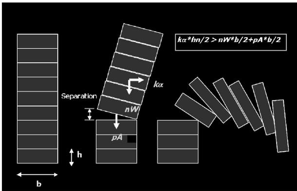
Fig. 10. Collapse mechanism of adobe buildings.
