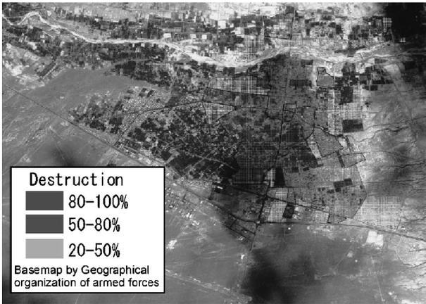
Fig. 1. Distribution of damage to buildings in Bam City [2].
