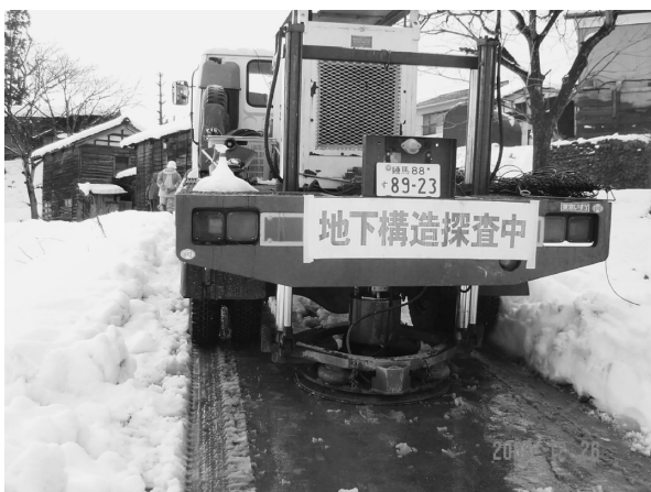
Fig. 2. A mini-vibrator truck (IVI, T-15000) used in the seismic profiling.
