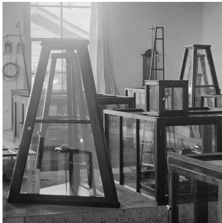
Fig. 2. Duplex pendulum seismometers (front left and far right) installed in the former Seismological Institute of the Tokyo Imperial University (the University of Tokyo) at Hongo.
