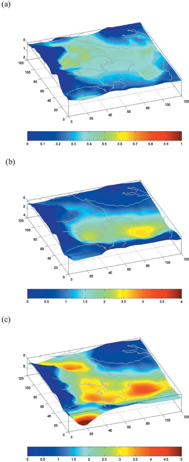
Fig. 3. The depth of (a) Shimsa/Kazusa, (b) Kazusa/Miura, and (c) Miura/Bedrock interfaces for the integrated 3D velocity-structure model (after Tanaka *et al.*, 2005). Contour bars indicate kilometers in depth.
