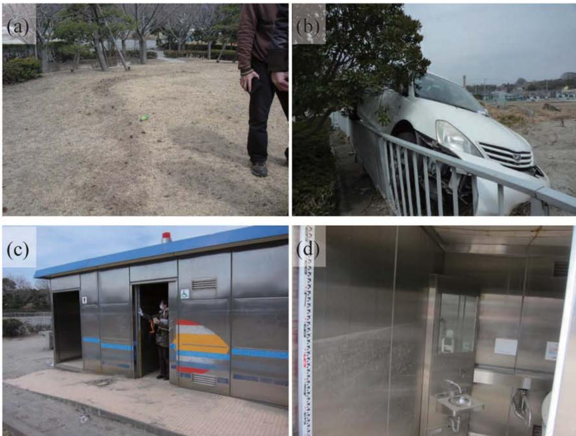
Fig. A274. (a) Trace of tsunami inundation limit on a hill at Nagisa Park. (b) Drifted car that crashed against a fence at Nagisa Park. (c) Public lavatory in Nagisa Park (tsunami trace survey point). (d) Watermark on an inner wall of the public lavatory (1.52 m above ground level, B25).
