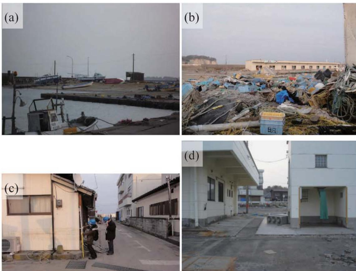
Fig. A258. (a)-(b) Damage at the Port of Kawajiri. (c) Tsunami trace survey point near the port. Watermark remaining on a wall of a house (1.13 m above ground level, B14). (d) Watermark on a wall of a building (1.87 m above ground level, B15).
