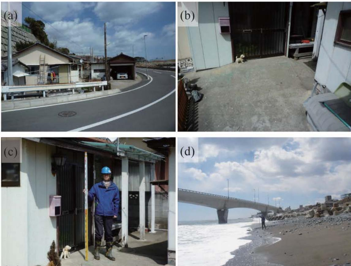
Fig. A264. (a) Mr. Seya's house in Higashicho (tsunami trace survey point). (b) Tsunami inundated near the entrance sliding doors. (c) Tsunami trace survey point in front of the entrance doors of Mr. Seya's house (B18). (d) Measuring ground height at a survey point based on the water surface of sea.
