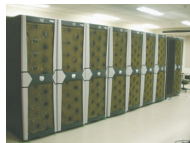
Fig.3 SGI Altix 4700 Computer system for the national joint research. We introduce the high-speed parallel computer system, and offer it to the national earthquake and volcanic researchers. In order to respond to increasing calculation demand, it is renewed in three SGI Altix 4700 systems which consists of 256, 160 and 16 cores from March, 2007. Annual registrants are about 450 persons and about 140 persons are utilizing actually every months. About 30~40% persons are researchers of university and laboratory except for the ERI. and, this system is utilized for the various research by many national researchers.
