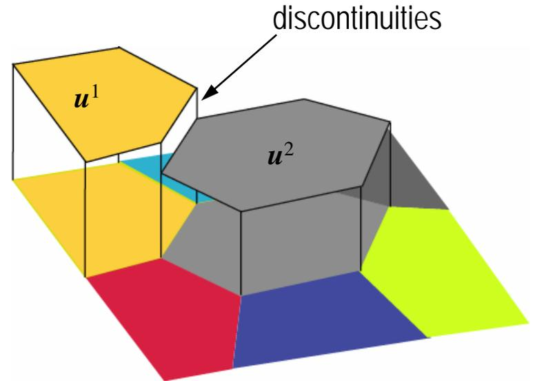
Particles can be interpreted as non-overlapping shape functions
