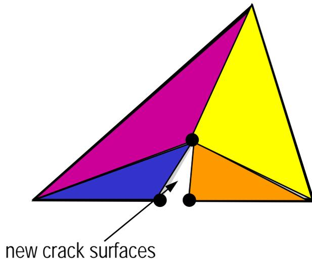
One new node and four elements are introduced
