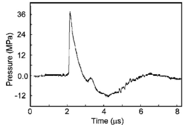
Typical pressure history in water induced by a single ultrasonic pulse
