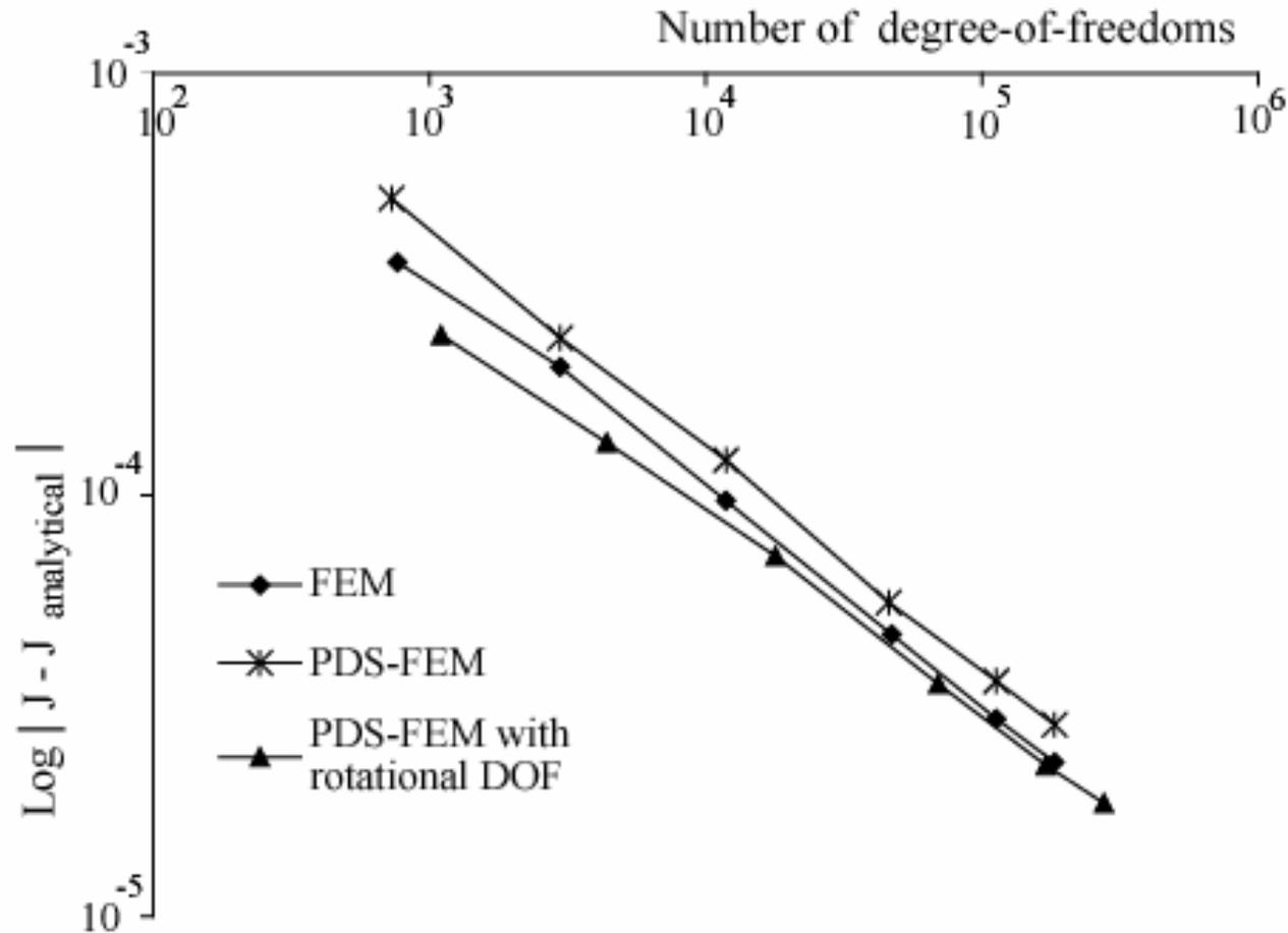
PDS-FEM crack tip stress field is as accurate as the FEM solution, regardless of approximate failure treatment. The accuracy of crack tip stress field can be improved by including rotational DOF
