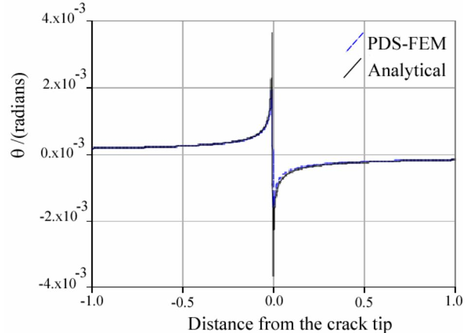
PDS-FEM estimates the rotational component fairly accurately, leading to better estimation of crack tip stress field
