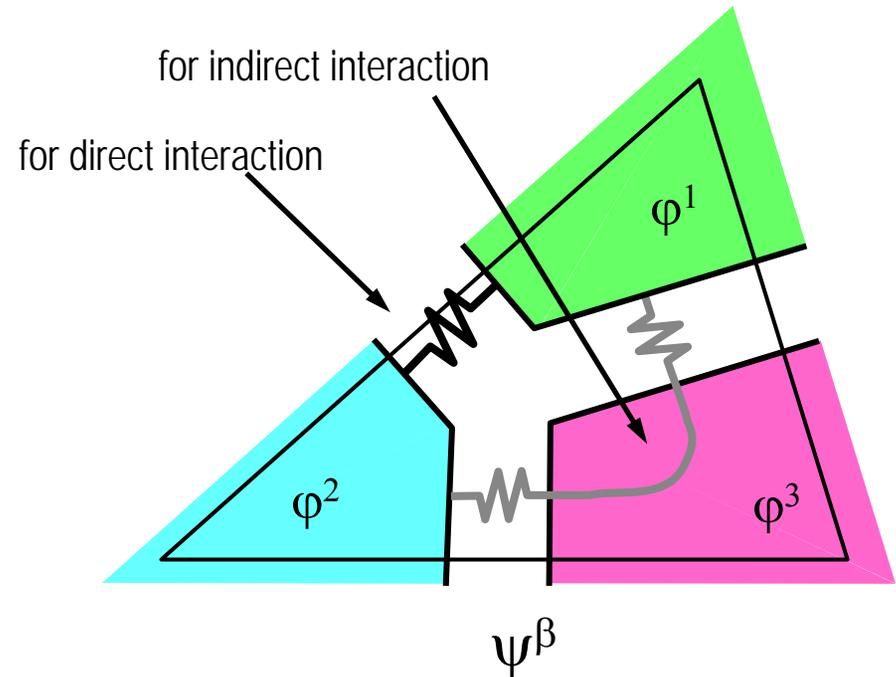
Failure is modeled by appropriately modifying the components of element stiffness matrix
