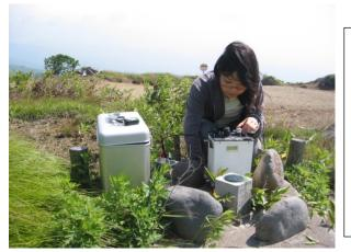
A Lacoste & Romberg gravimeter beside a levelling benchmark. It takes 5 to 20 minutes to finish a measurement, depending on operator's skill and experience.
