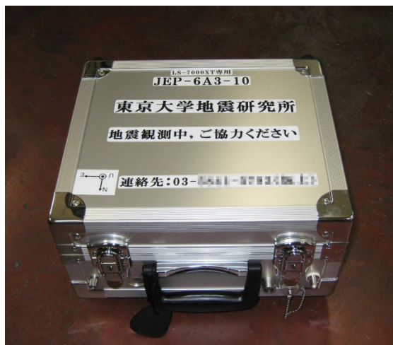
Portable strong motion observation system
