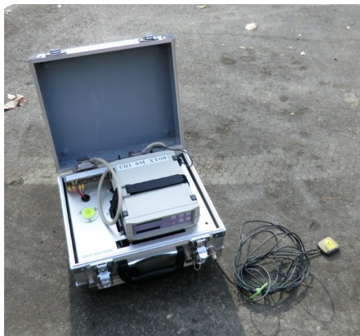
Portable strong motion observation system
