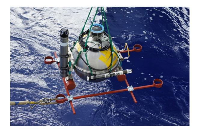
A vertical cylinder case at the left center is a body of the 3D current profiler.
