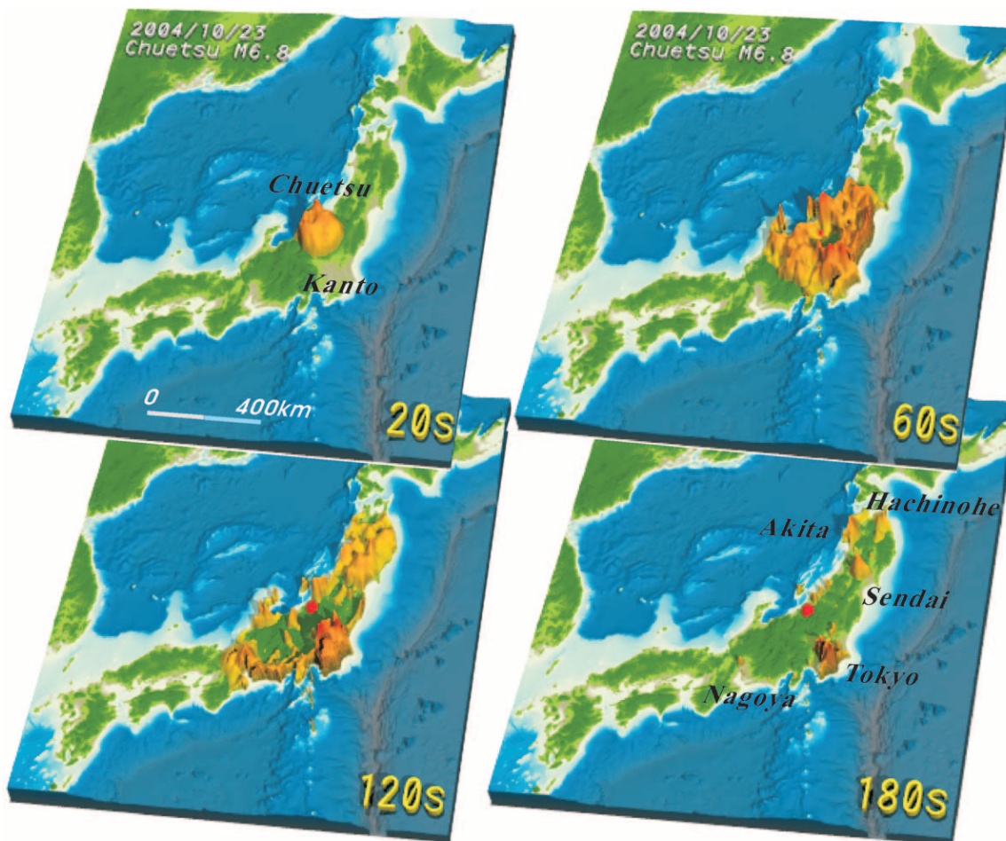
Figure 2. Distribution of ground motions following the Niigata-ken Chuetsu earthquake, Japan. The amplitude of the ground-velocity motions are shown for times of T = 20, 60, 120, and 180 sec after the earthquake rupture. (© See supplemental material in the online edition of BSSA.)
