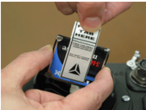
Figure 4 - 4 Only handle the drive by its side
