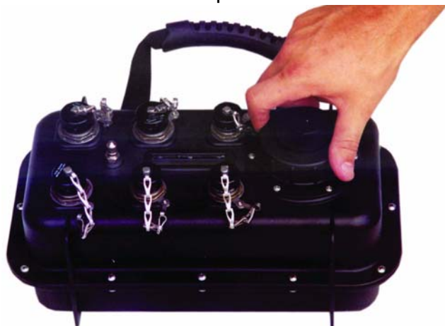
Figure 4 - 1 Remove cap from the well
