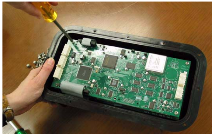
Figure 4 - 18 Loosen stack screws
