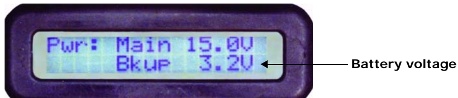
Figure 4 - 10 Backup battery voltage on LCD display
