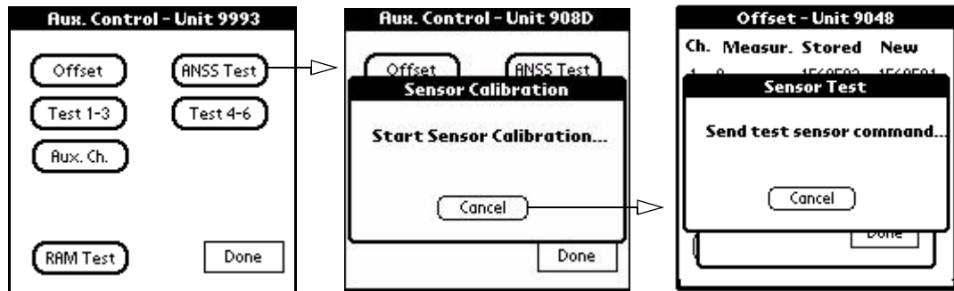
Figure 2 - 49 Send the internal accelerometer a test signal
