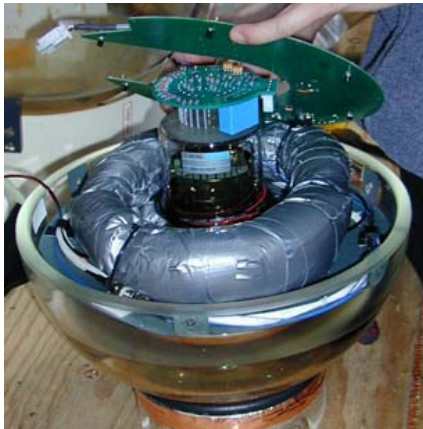
Digital Optical Module (DOM) 10inch PMT+ electronics
