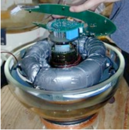
Digital Optical Module (DOM) 10inch PMT+ electronics
