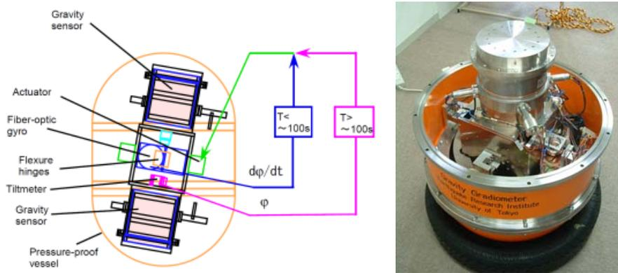
Fig. 13 Left: Schematic diagram of the feedback system of the forced gimbal. Two feedback loops are included; at high frequencies ( $\sim 100$ s), a gyroscope is used to reduce instant rotation through feedback circuit, while verticality is obtained at low frequencies ( $> \sim 100$ s) from a tiltmeter. Right: A two-dimensional forced gimbal installed in a pressure vessel.
