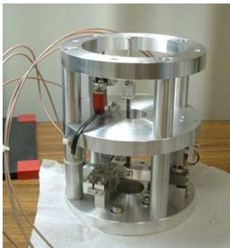
Fig. 12 A developed accelerometer as a gravity sensor.
