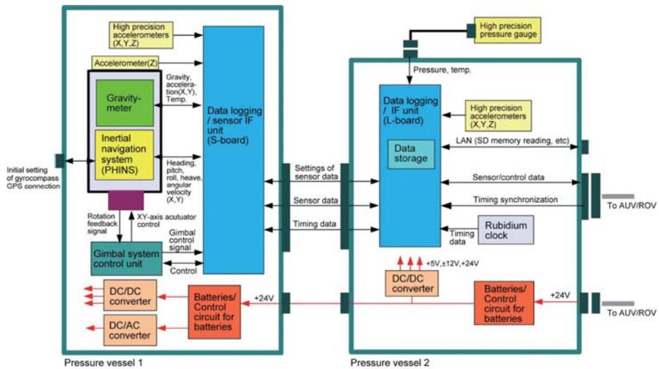
Fig. 8 Systematic diagram of the gravimeter system.
