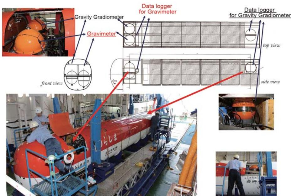
Fig.15 Layout of the system on the URASHIMA
