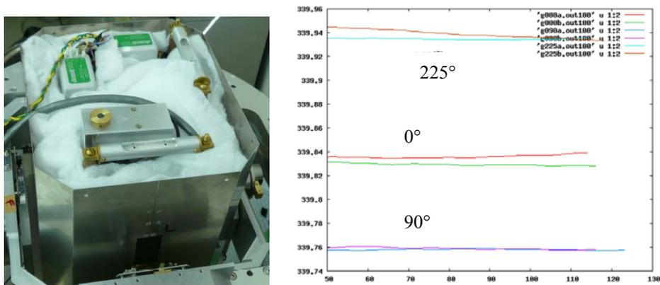
Fig.7 The permaaloy case contains the gravity sensor and DC servo motors for the gimbal system.
