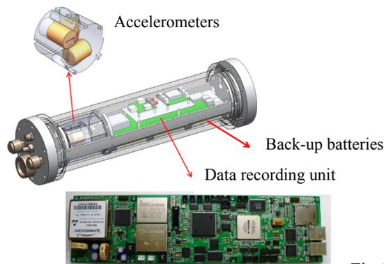
Fig 10. Data acquisition unit.
