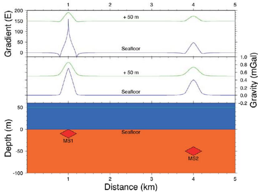
Fig.2 Estimated gravity (middle) and gradient (upper) variations are on a model (bottom). The model has two same shape deposits, MS1 and MS2, which have density differences of  $1\text{g/cm}^3$  against background.
