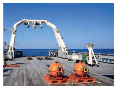
▲観測船上で投入を待つ長期観測型海底地震計 Long-term pop-up type ocean bottom seismometers on the deck of research vessel (Hakuho-maru) were waiting for deployment (October, 2014).
