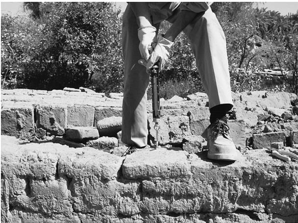
Photo 5. Measuring tension strength of mortar of sun-dried bricks.
