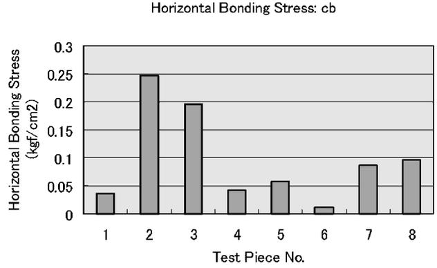
Fig. 7. Bonding strength in cross-section direction for baked bricks.
