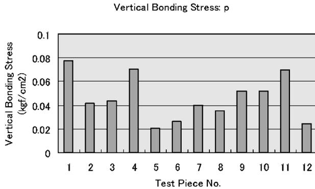
Fig. 6. Bonding strength in the vertical direction (tension) for sun-dried bricks.
