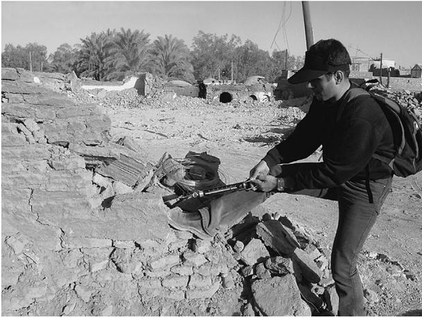
Photo 4. Measuring shear strength of mortar of sun-dried bricks.
