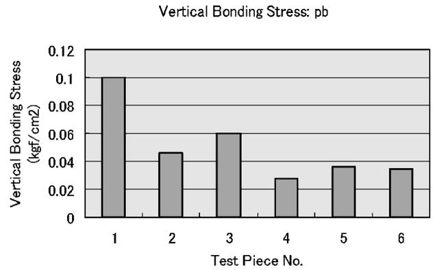
Fig. 8. Bonding strength in tension direction for baked bricks.
