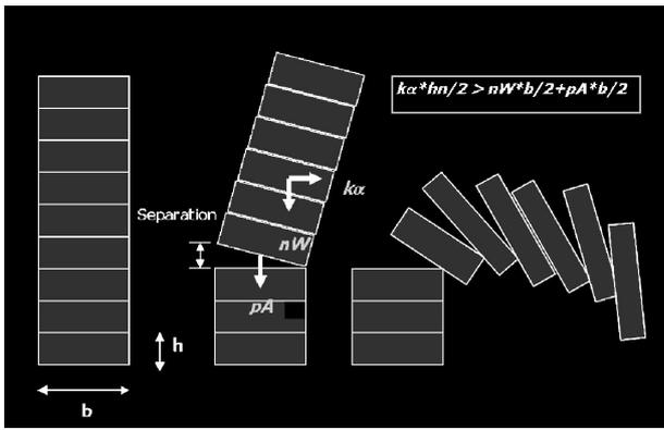
Fig. 10. Collapse mechanism of adobe buildings.
