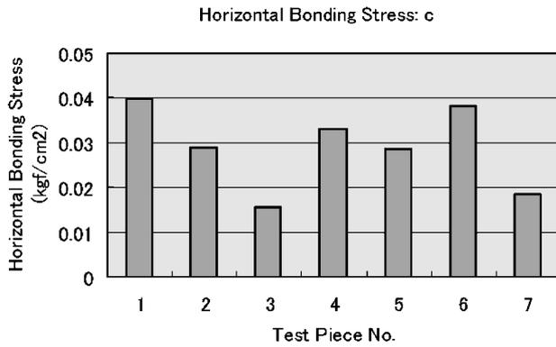
Fig. 5. Bonding strength in the horizontal direction (shear) for sun-dried bricks.
