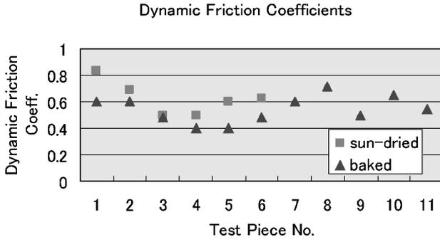
Fig. 4. The coefficient of friction for sun-dried (rectangular) and baked bricks (triangle).
