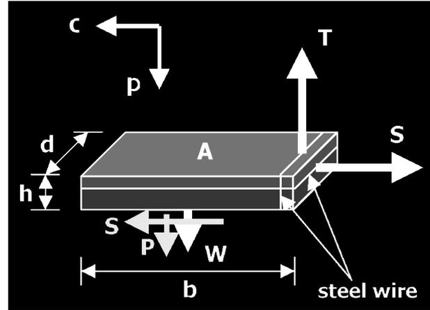
Fig. 3. Shear and tension strength estimation method.
