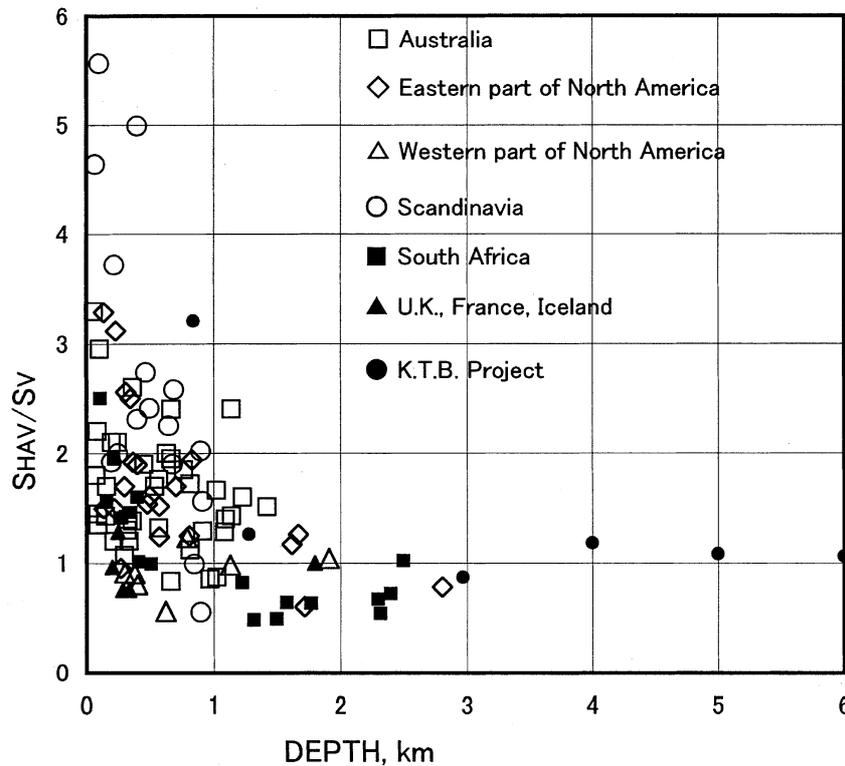
Fig. 8. Ratio between mean horizontal stress ( $S_{HAV}=(S_H+S_h)/2$ ) and overburden stress ( $S_v$ ) increases ground surface approaches. Based on the figure of Brown and Hoek [1978], KTB result [Brudy *et al.*, 1997] is added. In the original figure, data for North America were classified in two groups, data in Canada and those in the U.S.A. In this figure, the data for North America are classified into data for the eastern and western parts of the North American continent.
