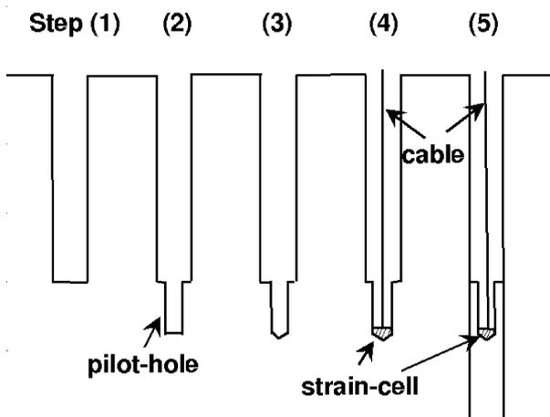
Fig. 1. General procedure of over-coring method. In step 1, a borehole is drilled to the depth of the measurement position with a scale of over-core size. In step 2, a pilot hole is drilled, and in step 3, the bottom of the pilot hole is ground to a semi-spherical or conical shape for borehole bottom measurement. In step 4, a strain-cell is embedded inside the borehole or glued to the bottom. In step 5, the pilot hole is over-cored.
