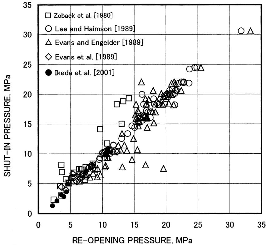
Fig. 4. An example of the relationship between the re-opening pressure ( $P_r$ ) and the shut-in pressure ( $P_s$ ) obtained in the U.S.A., Canada, and Japan. Many results indicate the relationship,  $P_r = P_s$ , which suspiciously shows that  $(S_H + P_p) / S_h$  is equal to 2.0 at any depth around the world.
