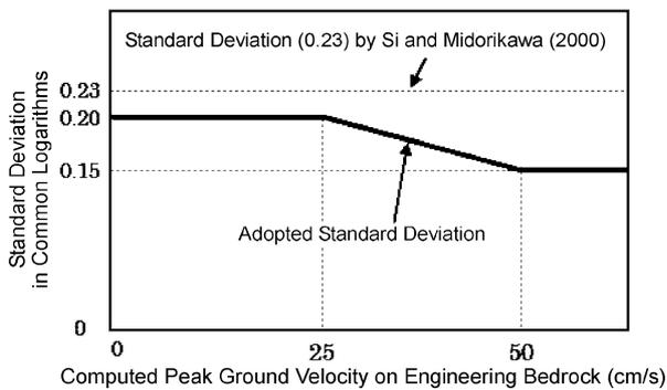
Fig. 8. Deviation model adopted in seismic hazard project (Earthquake Research Committee, 2005b)
