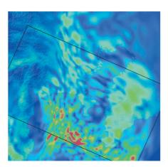
Fig. 5. Snapshots of simulated ground velocities for source model B of the 1923 Kanto earthquake with the integrated velocity model in the Tokyo metropolitan area. (a), (b), and (c) are 10, 20, and 40 seconds after rupture initiation.
