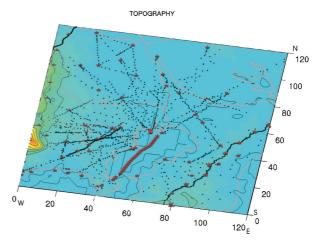
Fig. 2. Refraction/reflection survey used for integrating velocity model. The Boso peninsula, Tokyo bay, Sagami, and Kanto West lines with dense points are performed by the DaiDaiToku project.
