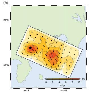
Fig. 1. Slip distribution of the 1923 Kanto earthquake from joint inversions of the strong motion, teleseismic, and geodetic data. (a) Model A by Kobayashi and Koketsu (2005) along the previous geometry of the Philippine sea slab. (b) Model B shown in Sato *et al.* (2005) along the new geometry of the slab.
