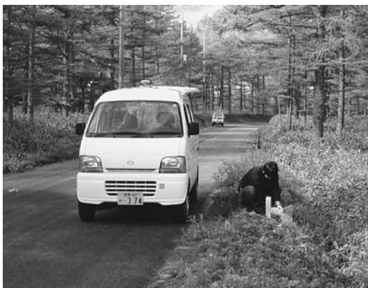
Fig. 3. An installation of the station. Light vehicle was preferable for deploying stations. GPS antenna was set on the roof of the vehicle and GPS receiver was running continuously during whole daily operations in the array.
