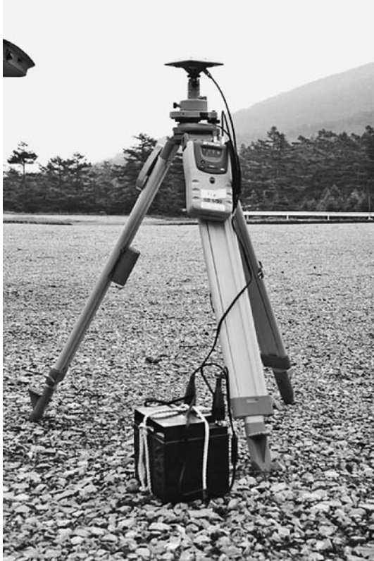
Fig. 2. The reference station for the positioning during daily installations.
