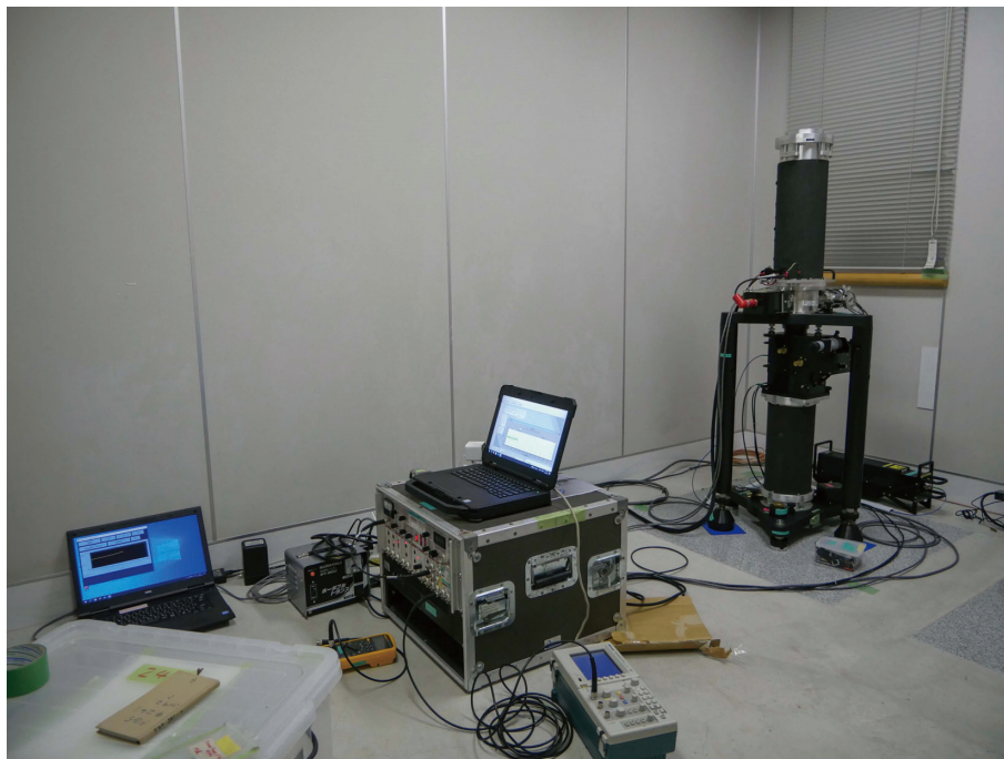
Fig. 2. Absolute gravity measurements with FG5 #241 at MFRI-E in September 2022. To the left, the precise barometer Paroscscientific 1000-16B (serial number #81465) can be seen.
