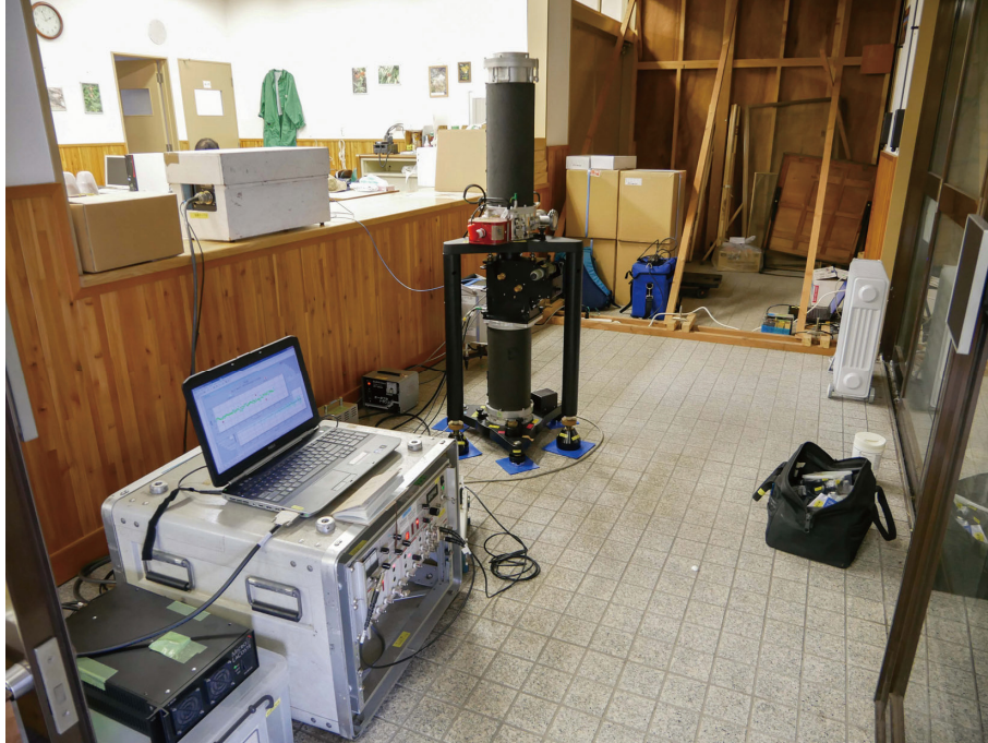
Fig. 3. Absolute gravity measurements with FG5 #109 at SL5ST in Mt. Fuji 5th Station Administrative Office, Road Public Corporation, Yamanashi Prefecture in September 2022.
