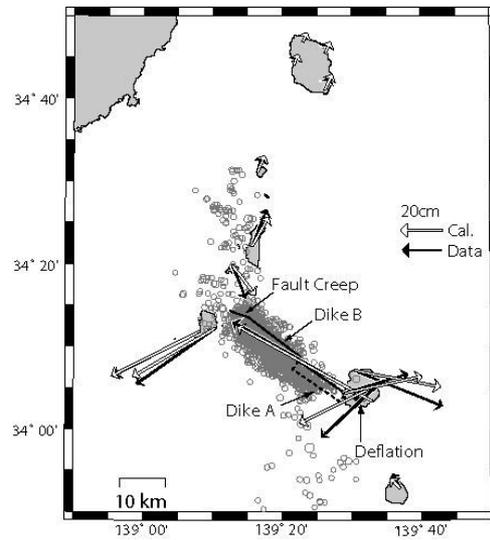
Fig. 3. Optimal fault model of ground deformation that accompanied the Miyakejima 2000 eruption. White and black arrows indicate calculated and observed displacements. Open circles are epicenters of earthquakes ( $M \geq 3.5$ ) (Nishimura *et al.*, 2001).
