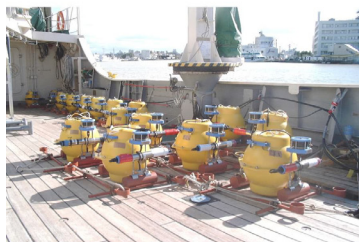
High-sensitive OBS (17" glass sphere)
