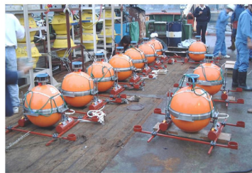
Long-term OBS (50-cm titanium sphere)
