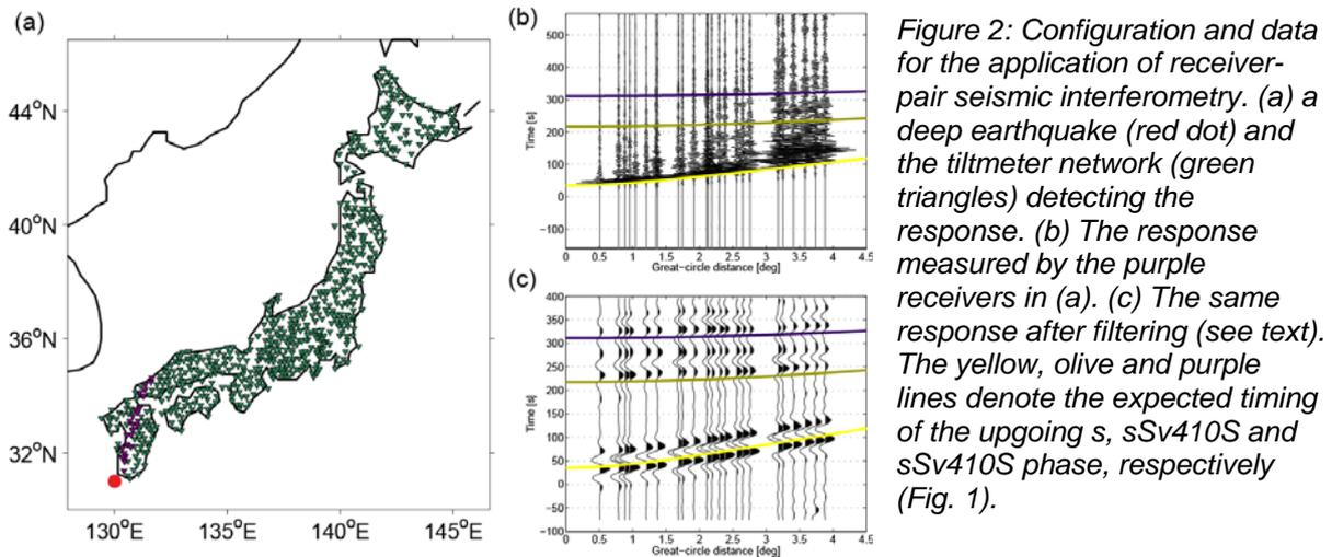
Figure 2: Configuration and data for the application of receiver-pair seismic interferometry. (a) a deep earthquake (red dot) and the tiltmeter network (green triangles) detecting the response. (b) The response measured by the purple receivers in (a). (c) The same response after filtering (see text). The yellow, olive and purple lines denote the expected timing of the upgoing s, sSv410S and sSv410S phase, respectively (Fig. 1).
