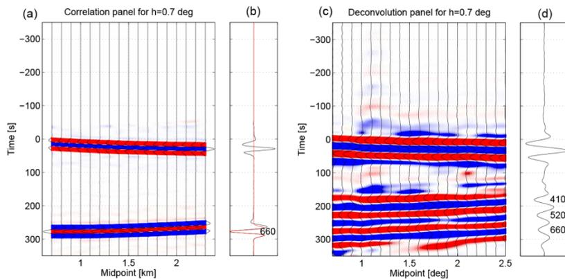
Figure 3: Results for applying RPSI on (a&b) numerical data and (c&d) field data, for a configuration as depicted in Figs. 1&2. The panels (a&c) show the results after the crosscorrelating step. The black traces (b&d) show the results after RPSI. For the numerical data a reference trace is provided (red trace in b).
