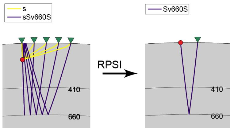
Figure 1: (left) From a deep earthquake (red dot) upgoing *s* (yellow rays) and the depth phase of the 660 reflection (purple rays) are recorded over an array of stations (green triangles). (right) By the application of receiver-pair seismic interferometry (RPSI) the response is extracted as if there were a source and receiver at the Earth's surface and the upside 660 reflection (purple ray) were measured.
