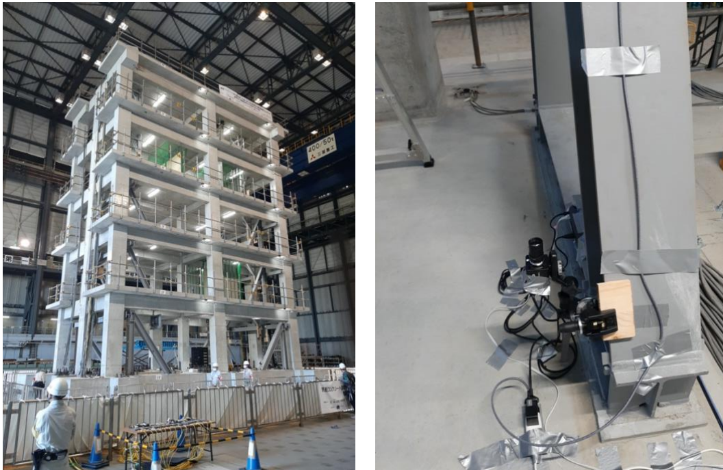
Figure 2: a) view of the specimen and b) installation of the DAD sensor at the first floor.
