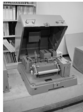
Fig. 6. SMAC-A strong motion seismograph (source: http://www.k-net.bosai.go.jp/KYOUKAN/ayumi/ayu5.htm ).
