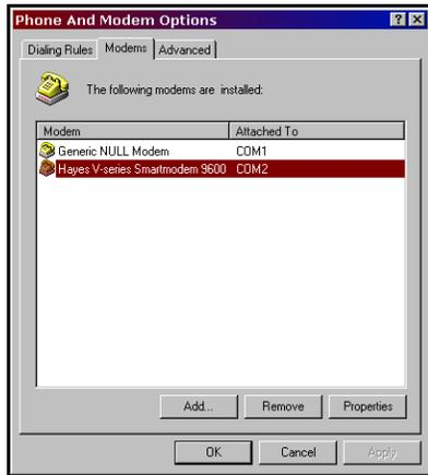
10. Select the **Properties** button to set the baud rate for the modem.
