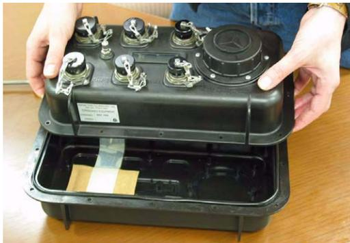
16. Bolt the two halves of the 130 DAS together using twelve #8-21x5/8 SS screws (Item 16) and #8 lock nuts (Item 17).
