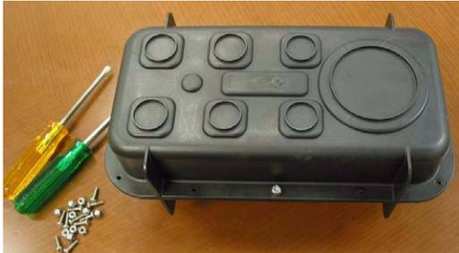
5. Unbolt the bottom base case (Item 15) of the recorder by removal of twelve #8-32x5/8 screws (Items 16) and the twelve #8 lock nuts (Item 17).
