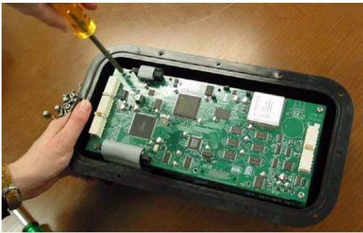
**Figure 58 Stack Screws**
