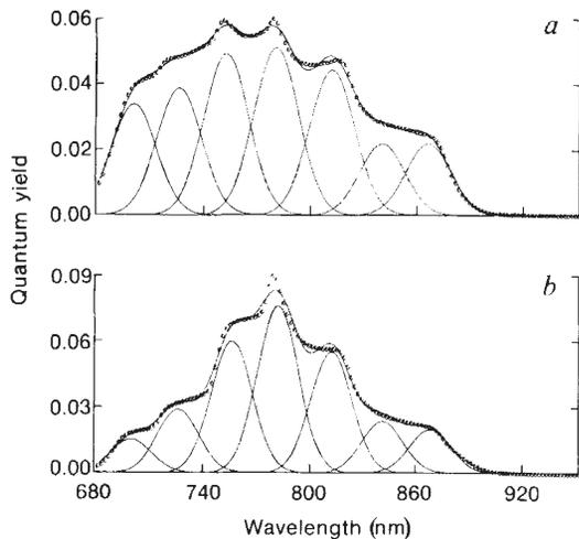
**Fig. 3** Photocurrent-wavelength spectra for GaAs/GaAs<sub>0.5</sub>P<sub>0.5</sub> SLS. *a* and *b* represent two different regions of the SLS wafer. Solid lines, theoretical fits to seven gaussian lines with equal linewidths.
