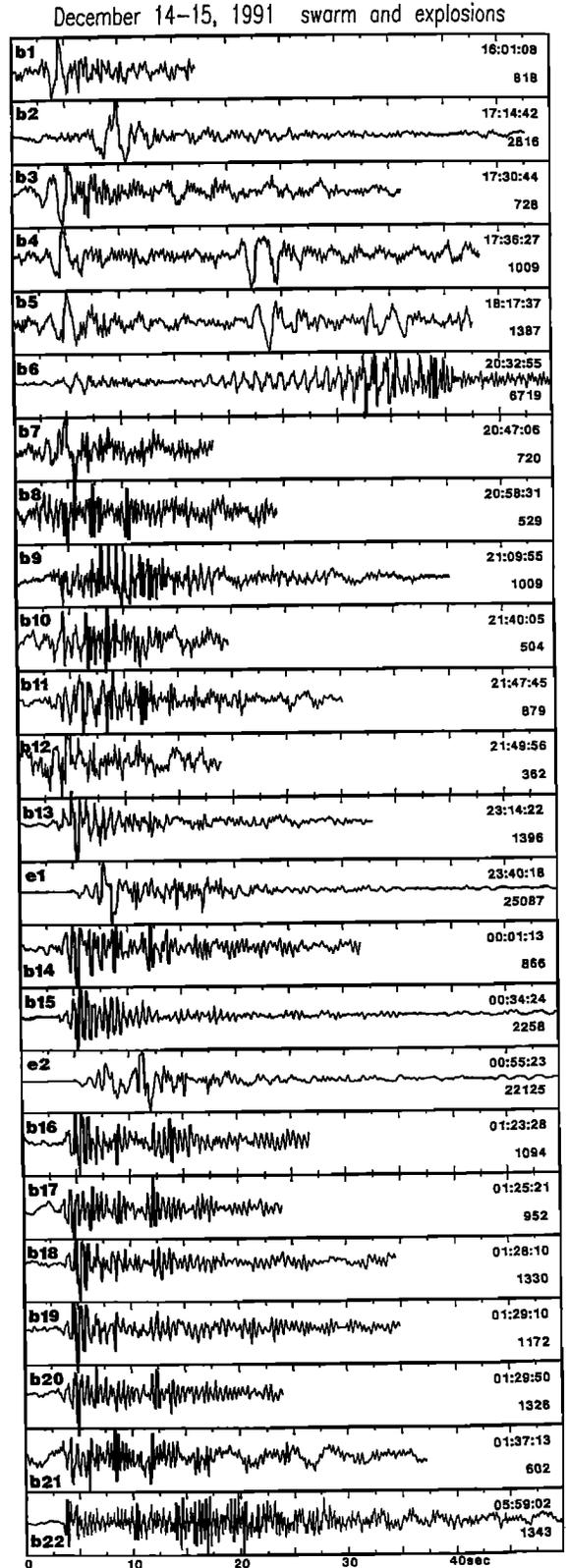
Fig. 3. Vertical velocity seismograms observed in an earthquake swarm. Origin times and peak-to-peak amplitudes (in  $10^{-8}$  m/s) are given at the upper-right and lower-right corners, respectively.
