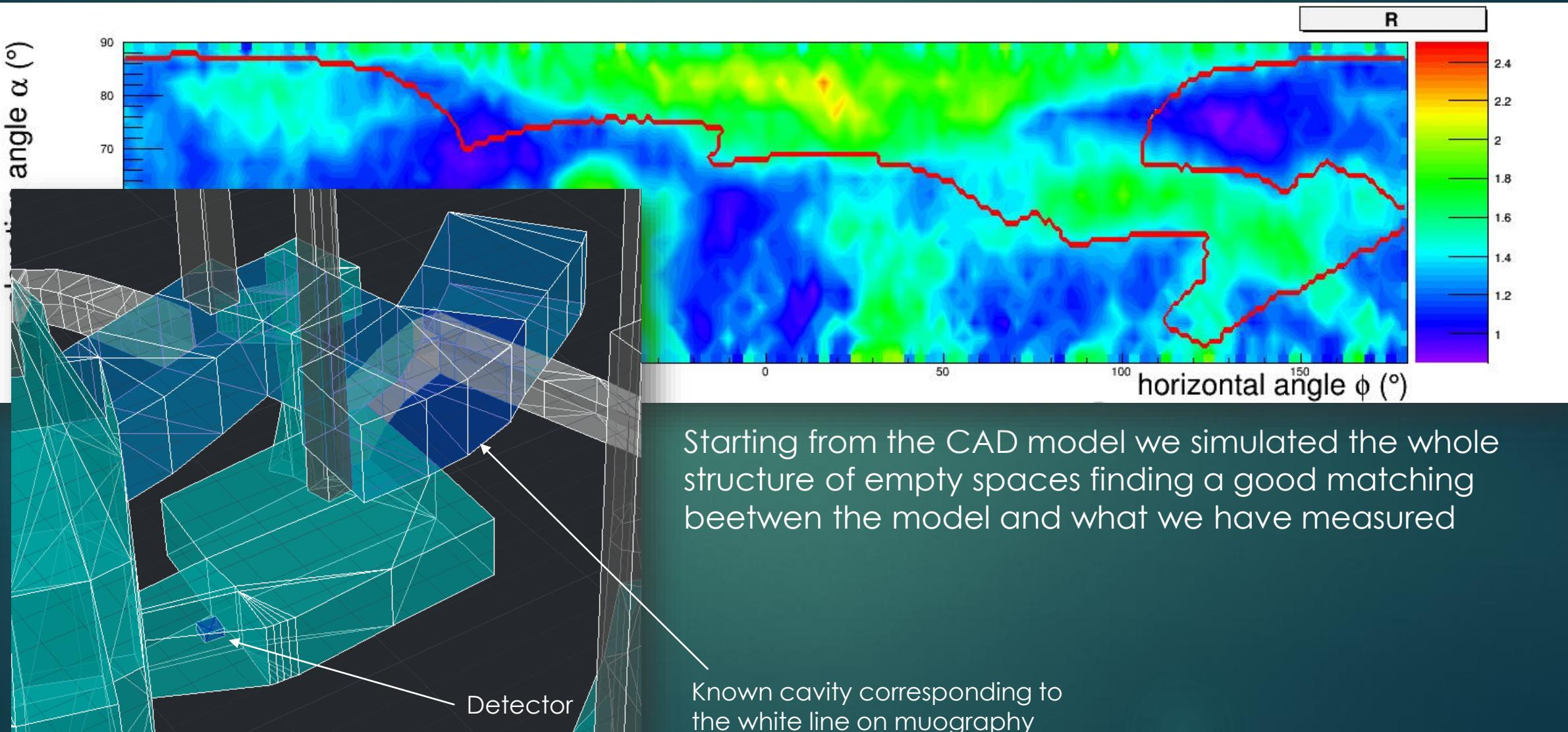
Starting from the CAD model we simulated the whole structure of empty spaces finding a good matching between the model and what we have measured
