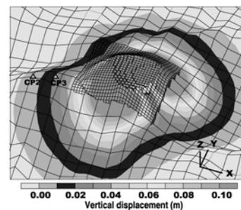
**Figure 4.** Contours of vertical displacement for a homogeneous volcano ( $E = 1$  GPa,  $\nu = 0.25$ ;  $\rho = 2600$  kg/m<sup>3</sup>) in response to removal of a dome volume of  $5 \times 10^6$  m<sup>3</sup>. Collapse scar shown in fine mesh. See color version of this figure in the HTML.
