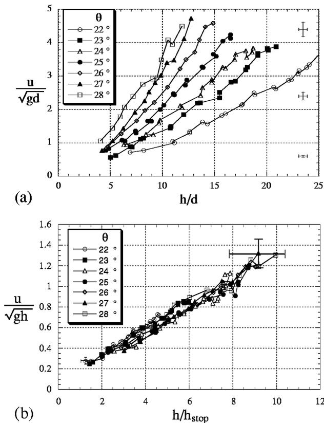
FIG. 4. (a) Dimensionless velocity  $u/\sqrt{gd}$  as a function of  $h/d$  for different inclination angles. (b) Froude number  $u/\sqrt{gh}$  as a function of  $h/h_{stop}(\theta)$  for different inclinations. Data obtained for system 1.
