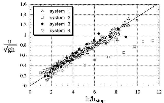
FIG. 5. Froude number  $u/\sqrt{gh}$  as a function of  $h/h_{stop}(\theta)$  for the four systems of beads and for different inclination angles.
