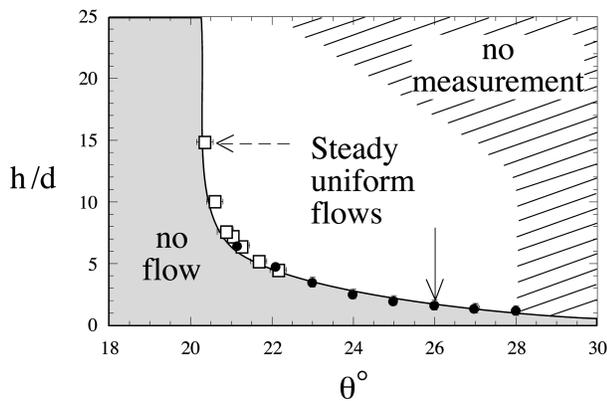
FIG. 2. Region of the parameter space ( $\theta, h/d$ ) where steady uniform flows are obtained; ●—measurements of  $h_{\text{stop}}(\theta)$ ; □—measurements of  $\theta_{\text{stop}}(h)$ . Some error bars are hidden by the symbols. Data obtained with system 1. Solid arrow (respectively, the dashed arrow) represents a typical evolution of the system in the parameter space during the measurement of  $h_{\text{stop}}(\theta)$  [respectively,  $\theta_{\text{stop}}(h)$ ].
