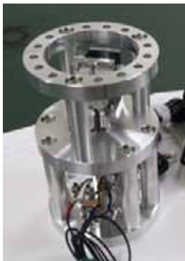
Fig. 9 A new accelerometer as a gravity sensor.
