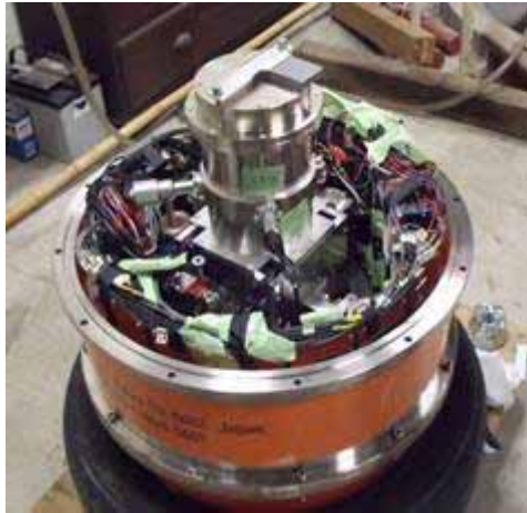
Fig. 10 A two-dimensional forced gimbal installed in a pressure vessel.
