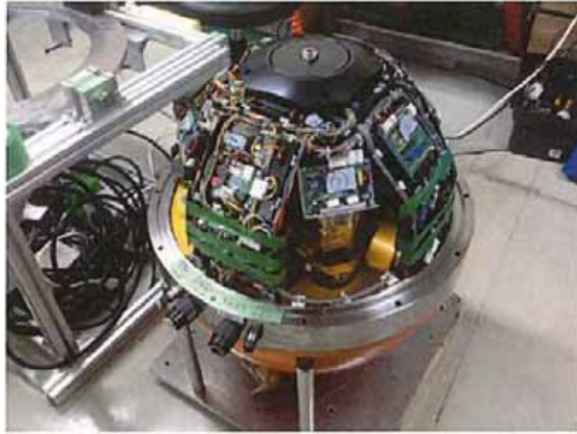
Fig.8 Photograph of inside of all-in-one type gravimeter
