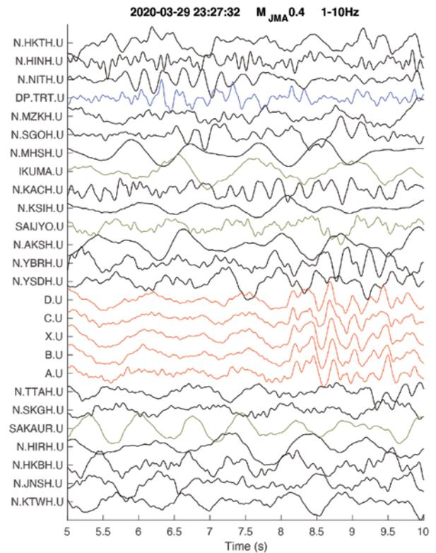
Fig. 1. Observed seismograms (A–D) and their stacked waveform (X).
