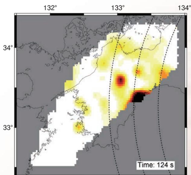
**Fig. 1.** Log-likelihood distribution at 124 s after the 2016 off-Mie earthquake. Darker colors indicate a higher likelihood of occurrence of a very low-frequency earthquake. Dotted black curves are approximate arrivals of the large-amplitude waves shown in Figure 2.
