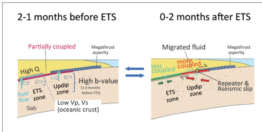
Fig. 1. Schematic cross-sectional views beneath the Kii peninsula before and after the occurrence of ETSs.
