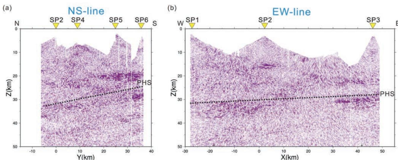
Fig. 2. Post-stack migrated depth section with shot positions denoted by inverted yellow triangles. Dashed lines indicate our interpretation of the top of the PHS. (a) N–S line. (b) E–W line.
