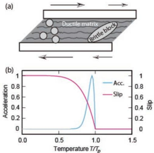
**Fig. 1.** (a) Schematic illustration of fault zone structure. (b) Simulated temperature dependence of slip (purple) and acceleration (blue).
