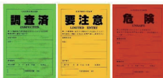
Figure 1: Green, Yellow, and Red tags for current Japanese rapid inspection, which is based on visual inspection by engineers.
